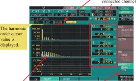
Inter-harmonics display Detailed numerical data for up to the 50th harmonic (light blue) order is displayed in a list.
